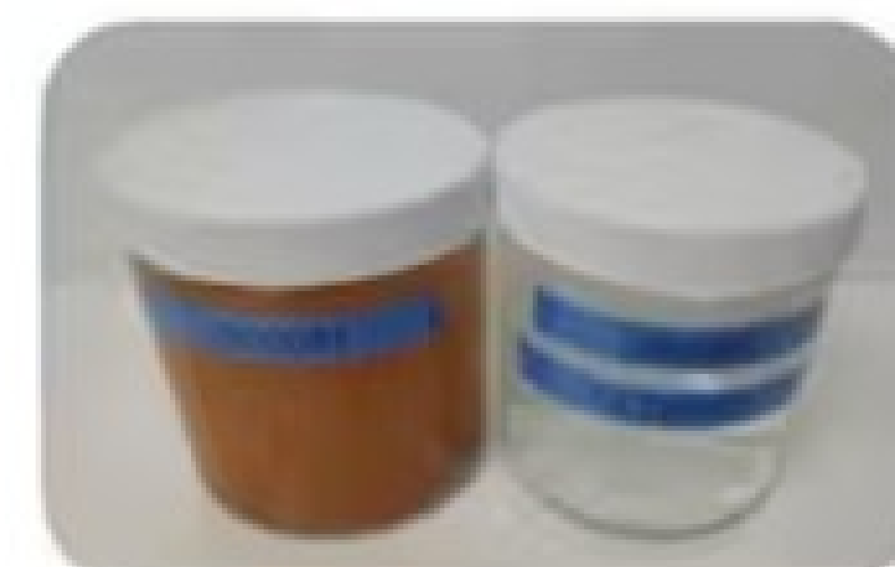
Image 2: DSU-H: Filter #001: Container on the left displays the backwashed water (unfiltered) while the container on the right (labeled "Filtered") displays the filtered water from the DSU-H filter.
