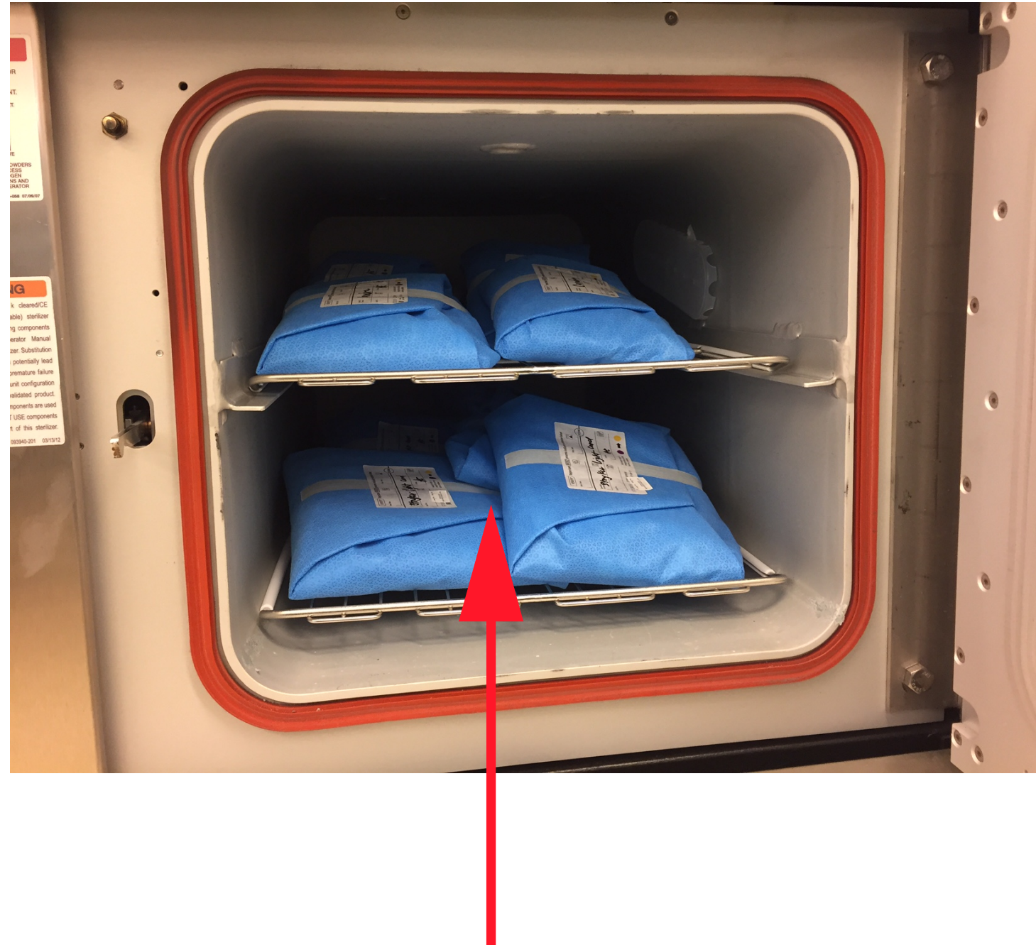
Overlapping packages in low-temperature gas plasma sterilization chamber
